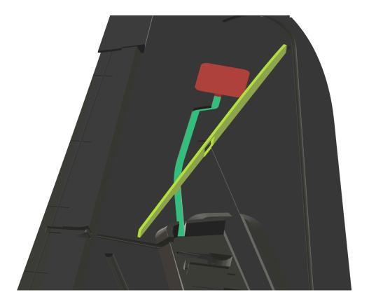
Next, install the servo bay plastic tray, and screw down the servos.
