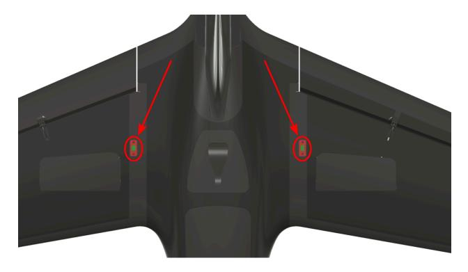
Connecting them is as easy as detaching them. Install the two carbon rods into the main body and slide the wings on them till the end. When done correctly, the push button will be flush.
