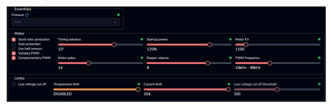
**Stuck Rotor Protection:** ON Startup power: 125% **Stall Protection:** OFF Motor KV: 1000 **Motor Poles:** 14 **Use Hall Sensor:** OFF Variable PWM: **Beeper Volume:** ON 8 **Complementary PWM:** ON PWM Frequency: 24-48KHz Timing advance: 15° **Temperature Limit:** OFF **Current Limit:** 204 Low voltage cutoff: OFF
