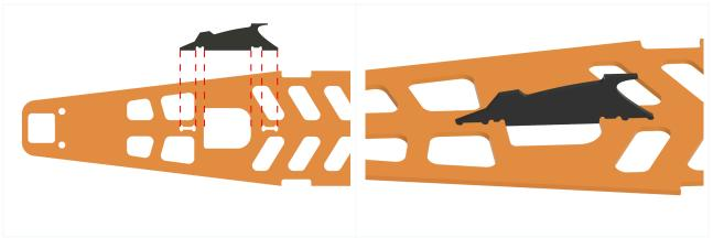
Then, wrap the velcro straps around the base plate and glue the base plate in place. Avoid glue in the pockets for the velcro strap - that way, it can be replaced later if necessary.
