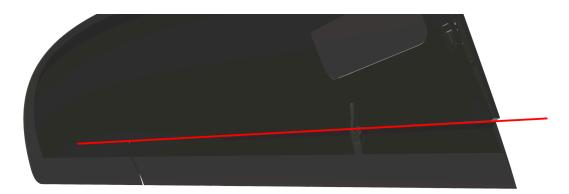
Install some double-sided tape on both surfaces. The tape must be as wide as half of the final filament tape. Then, add the filament tape over it while moving the elevon down close to 90° and press it firmly.
