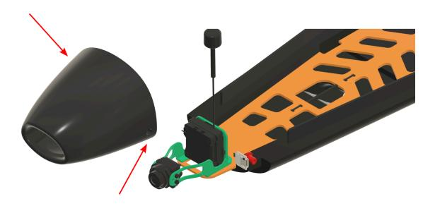
For the antennas, just poke a small hole through the foam of the main body, about 1-2cm in.
