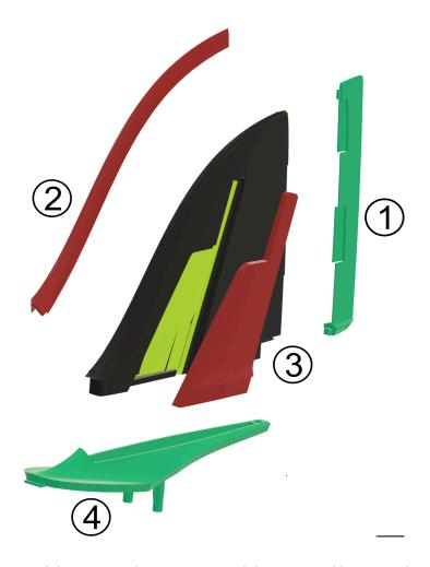
When just gluing the bottom of the antenna bay cover (3) and then covered by some clear tape or just slightly glued in on the rest, the cover can be removed to change the antenna or later installation.
