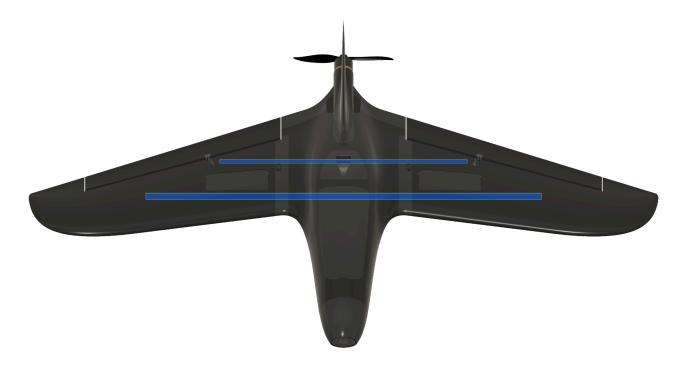
Two carbon rods reinforce the wings inside. Install them by sliding them into the designated guides.
