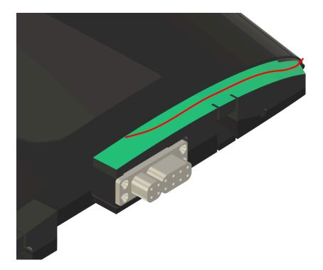
For the installation of the LED strip itself, cut the round edge at the notch along the wing front. On the vertical stabilizer, the surface is already flat. Glue your LED strip on the flat surfaces.
