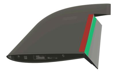
When down, the elevon should move without resistance. Reconnect the servo link and check the servo throw and center.
