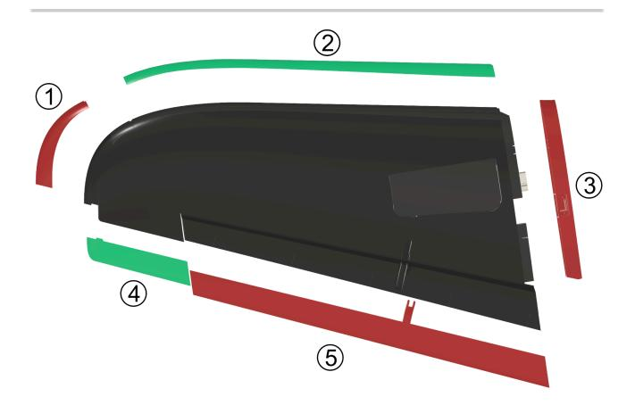
On the Elevons, make sure the notches align and that you use glue on the whole contact surface.
