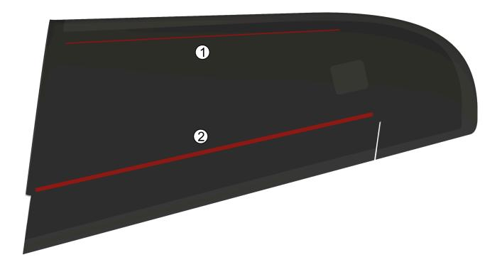
You need to run a wire from the edge to the wing connector to install the LED strips on the leading edge. Create a shallow cut for the cable (recommended), or simply press-fit it under the plastic wing connector and feed it into the servo bay to connect it to the electronic connector.
