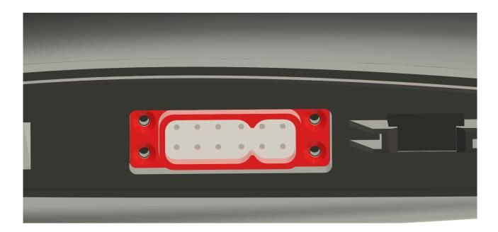
You can use the pins as you like. If you want to use the LED stripes in the wing edge and a VTX, you might need to use some pins for multiple devices. For example, using the same pin for 5V and GND for both servos allows for VTX (with CRSF) and LED, and both servos by just using 12 pins.
